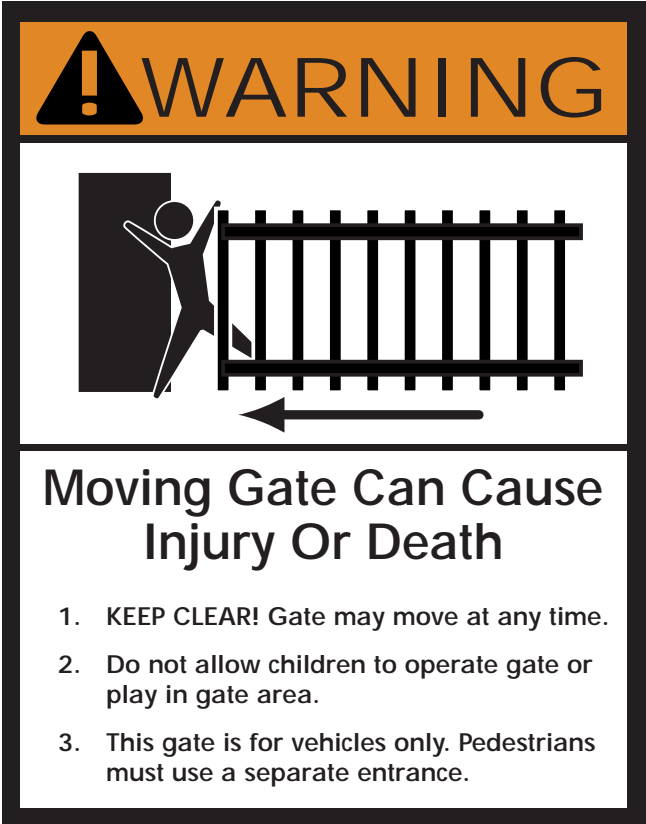
warning signs (2 enclosed) to be installed on each side of the gate (3–5 feet above the bottom of the gate)
